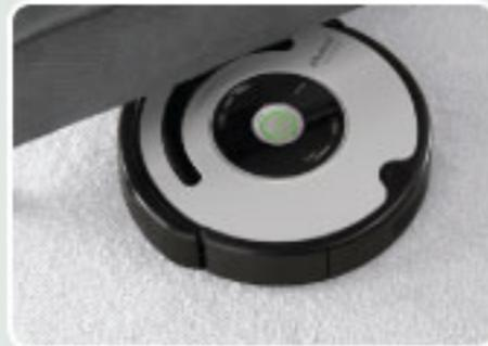
Cleans under and around furniture, using its light-touch bumper to gently touch and move around the obstacle.
