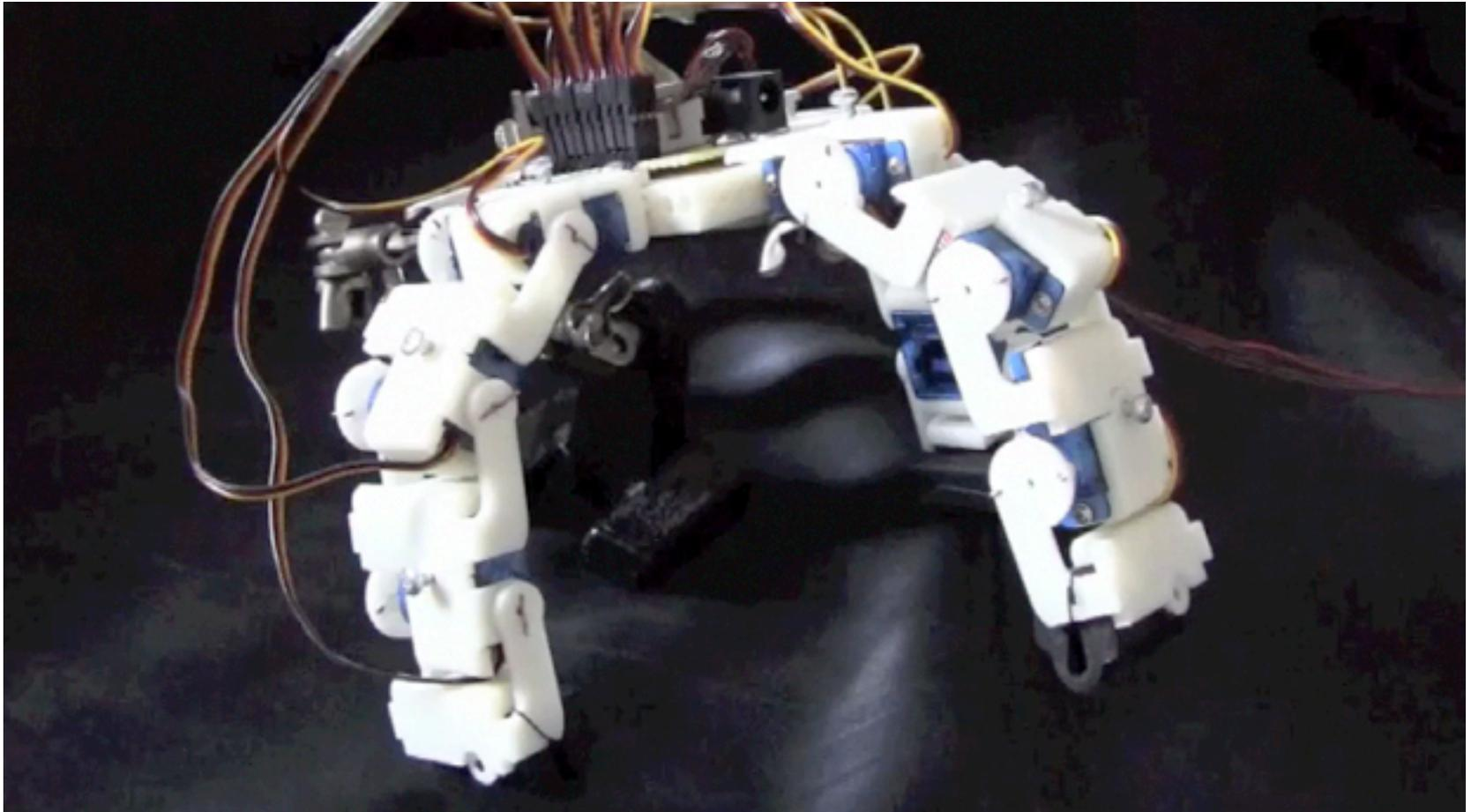
9 joints, (DoF) | 9 motors, | only 4 synergies (Degree of Control)
