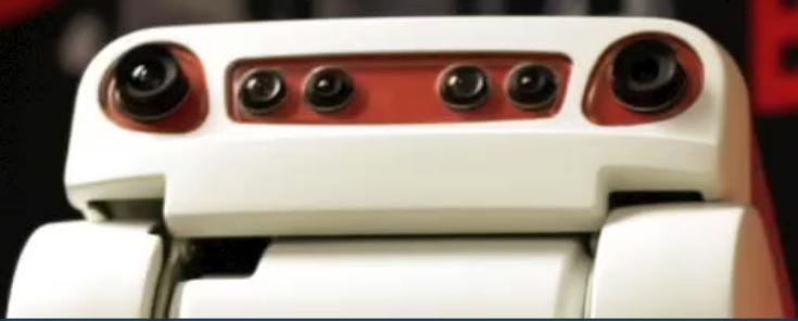
A close-up photograph of the head of a white PR2 robot. The head features two large black camera eyes on the sides and a central sensor array with four smaller black lenses. The background is a blurred red and black banner with the word "BOSCH" in red.
