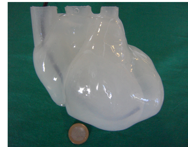
Figure 2: Cardiac phantom made of silicone with a shore hardness of 40. The silicone heart consists of two completely separated cavities that represent the heart chambers. An instrument was inserted into the right heart chamber through one of its three openings.
