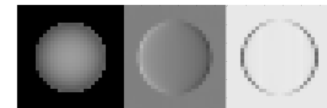
Figure 3: Absorption (left), differential phase-contrast (middle, DPC) and dark-field (right, DCI) images of an aluminum oxide sphere (diameter 1 \text{ mm} ) simulated with a detector pixel size of 50 \mu\text{m} . As the interferometer is only sensitive to phase shift and scatter in horizontal direction the signal at top and bottom of the sphere is weaker than on the sides in the two images on the right. The change in the gray values in the DPC image indicates that the wave front is shifted to different sides at the opposite sides of the sphere. Scattering occurs at the projected edges as can be seen in the DCI image.
