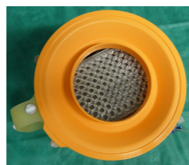
Figure 2: Neurosurgery phantom: a compact disc (CD) box with 18F-FET glued inside a mixing bowl; a 96 well microplate attached rigidly on the CD box, and filled with 18F-FET in pre-defined T/B activity ratios, simulating residual tumor among healthy brain tissue.
